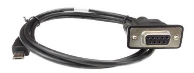
CBL003 is a 1 meter adaptor cable for connecting a PC running terminal emulation to VadaTech products that use a MicroUSB connector for RS-232 console I/O (e.g. for use with VadaTech AMCs).
