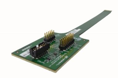
DA234 is a JTAG extender cable that enables standard JTAG pods to be used with VadaTech products fitted with a low profile ZIF connector. The flexible PCB is thin enough to fit between AMC, ATCA and VPX front panels.
