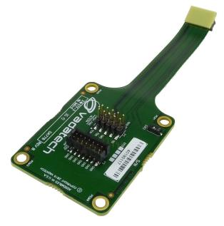
DA778 is a JTAG adapter cable that enables standard JTAG cables to be used with VadaTech JTAG Switch Module (JSM) or JSM-enabled products. The adapter breaks out the VadaTech proprietary JSM connector to a Xilinx or Altera/Intel FPGA JTAG header. It also includes a CFG DIP switch for use when the VadaTech JSM-enabled product does not have a CFG toggle switch on the front panel.
