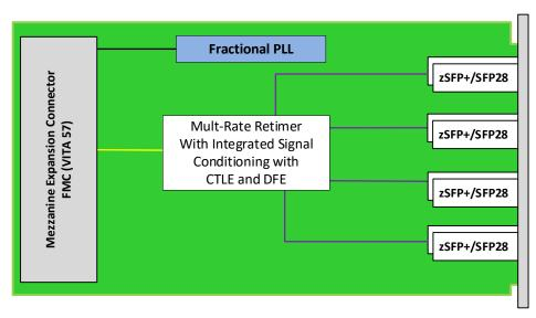
Figure 2: FMC116 Functional Block Diagram
