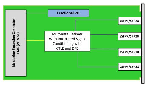
Figure 2: FMC117 Functional Block Diagram
