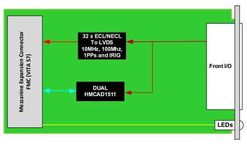
Figure 3: FMC152 Functional Block Diagram
