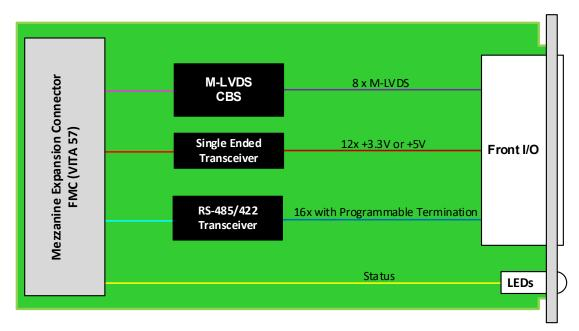
Figure 2: FMC156 Functional Block Diagram
