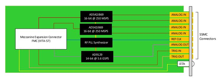
Figure 1: Block Diagram
