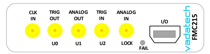
Figure 3: FMC215 Front Panel
