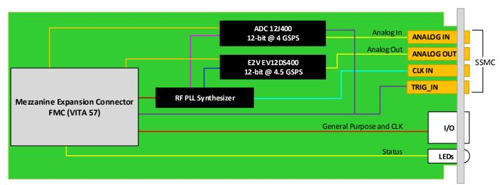
Figure 2: FMC215 Functional Block Diagram
