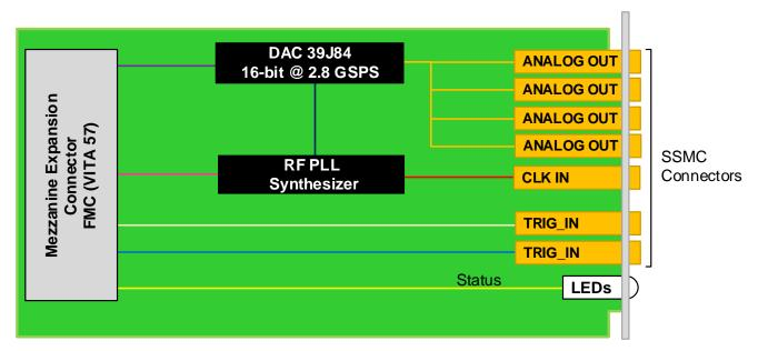
Figure 2: FMC224 Functional Block Diagram
