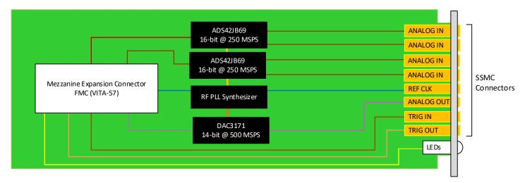
Figure 2: Block Diagram
