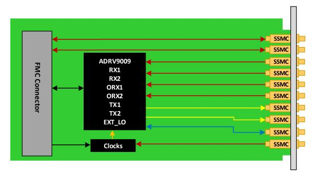
Figure 2: FMC238 Functional Block Diagram
