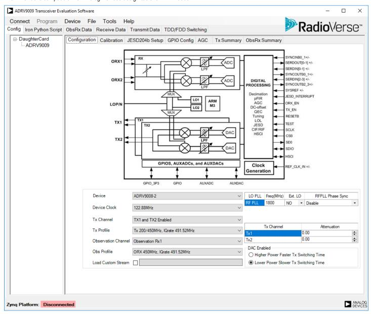
Figure 4: FMC238 Compatible Design Tools for ADRV9009
