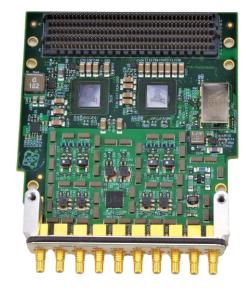
Figure 2: FMC249 Top View without Heatsink
