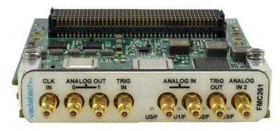
Figure 3: FMC261 Front Panel
