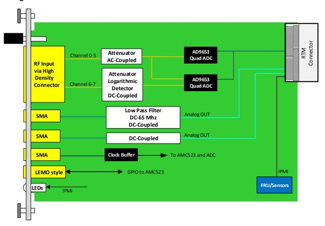
Figure 2: MRT523B Functional Block Diagram
