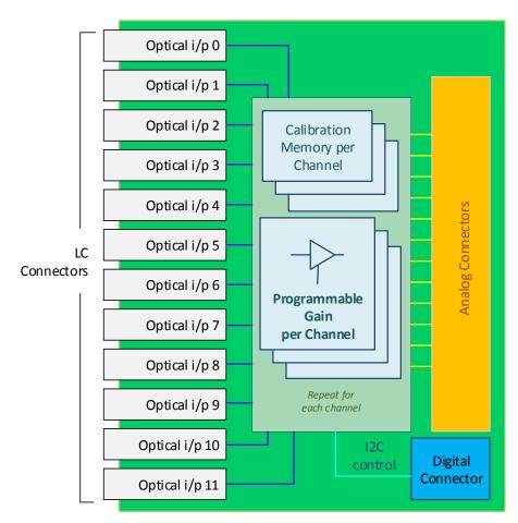
Figure 2: MZ523C Functional Block Diagram
