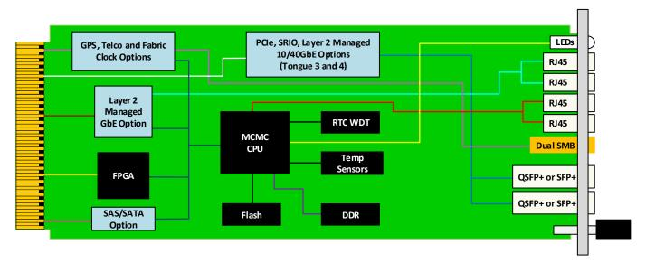
Figure 2: UTC002 Functional Block Diagram (SFP+ is used for 10GbE and QSFP+ for PCle/SRIO)
