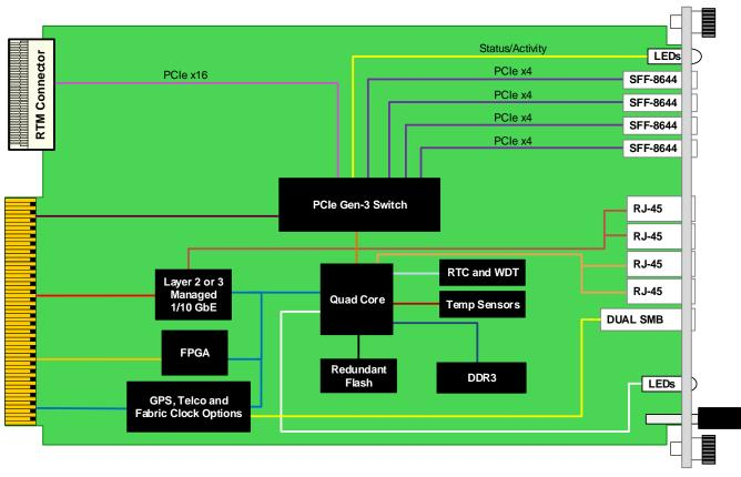
Figure 5: Block Diagram (PCIe Option)
