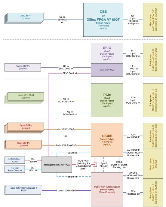
Figure 10: Block Diagram - Connectivity and Fabric Options
