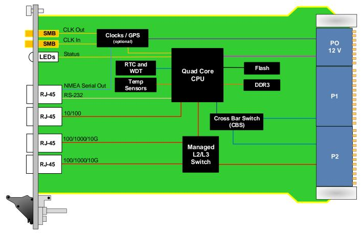
Figure 2: VPX006 Functional Block Diagram
