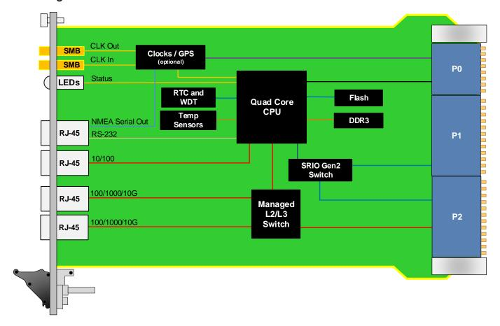
Figure 2: VPX008 Functional Block Diagram
