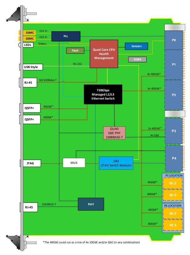
Figure 4: VPX011 Functional Block Diagram
