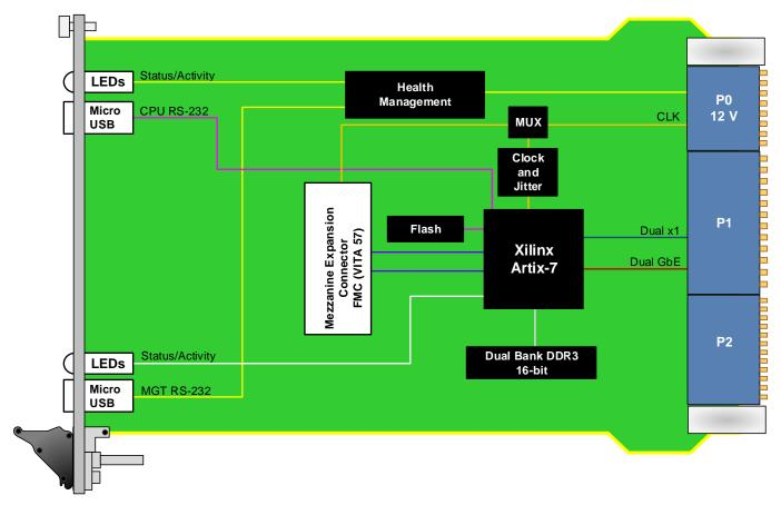
Figure 2: VPX519 Functional Block Diagram
