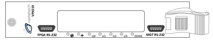
Figure 3: VPX519 Front Panel
