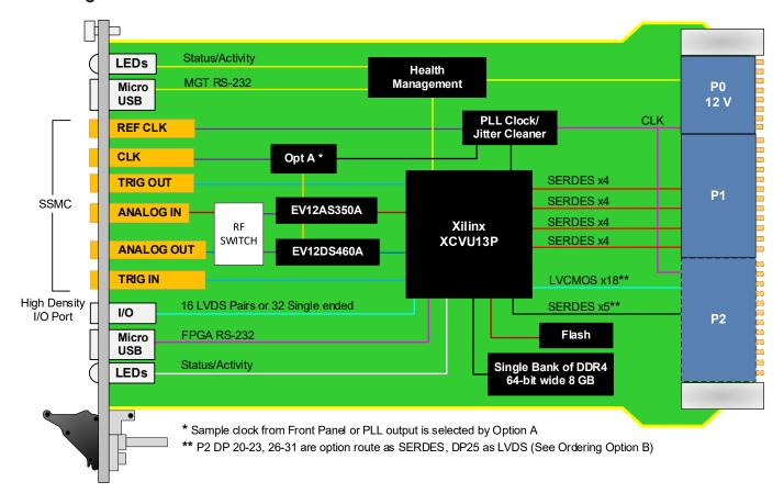
Figure 2: VPX570 Functional Block Diagram
