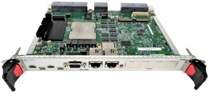
Figure 3: VPX763 without Heatsink
