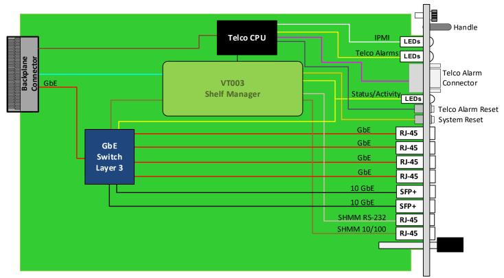
Figure 2: VT052 Functional Block Diagram
