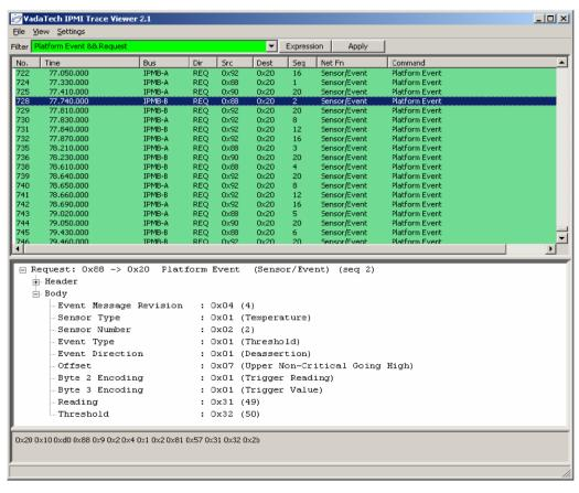
Figure 3: IPMI Protocol Analyzer Trace Viewer Output
