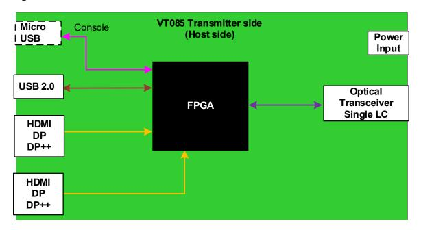
Figure 2: VT085 Functional Block Diagram
