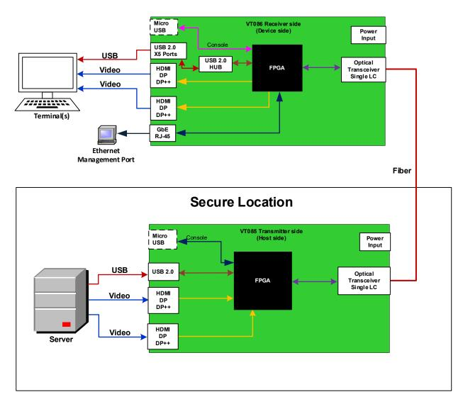
Figure 4: VT085/VT086 Connectivity Block Diagram
