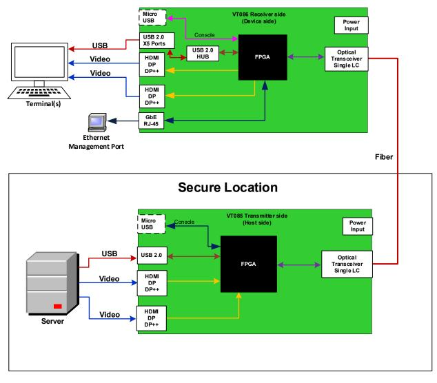
Figure 3: VT085/VT086 Connectivity Block Diagram
