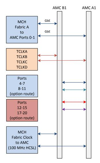
Figure 4: VT819 Backplane Connections
