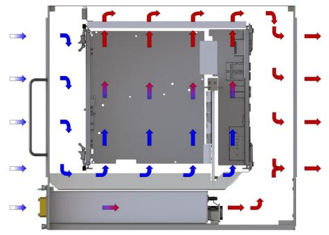
Figure 4: VT820 Cooling Airflow
