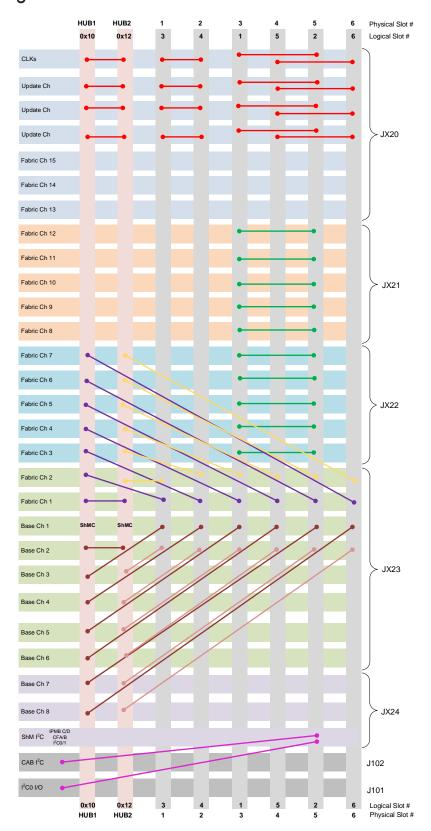
Figure 5: VT837 Backplane slot routing
