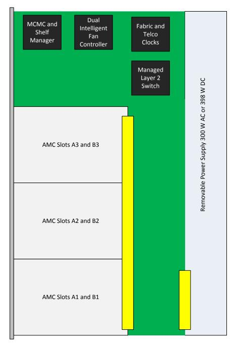
Figure 3: Top Level Block Diagram
