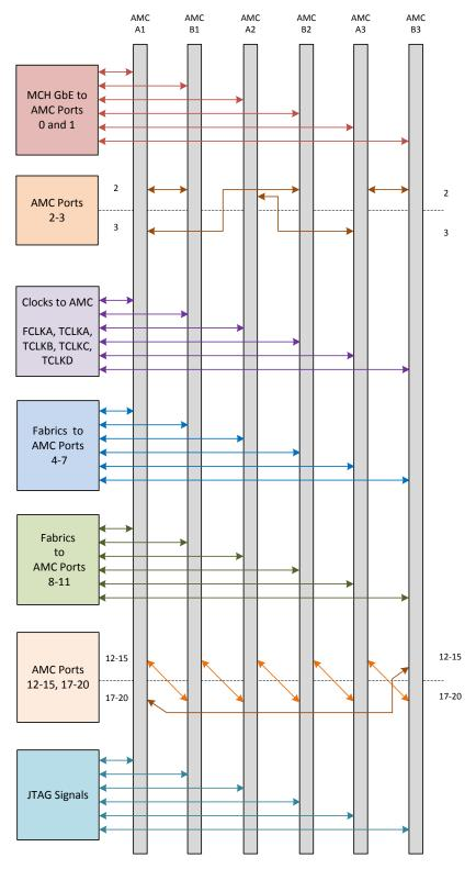
NOTE: Since the PCIe Fabric has 12 ports of x4 (48 lanes total) there is option to run all the ports as x8 ( on ports 4 to 11) or single dual x4. With the SRIO there are two options, SRIO x4 on all the ports 8-11 or on slots B2 and B3 only.
