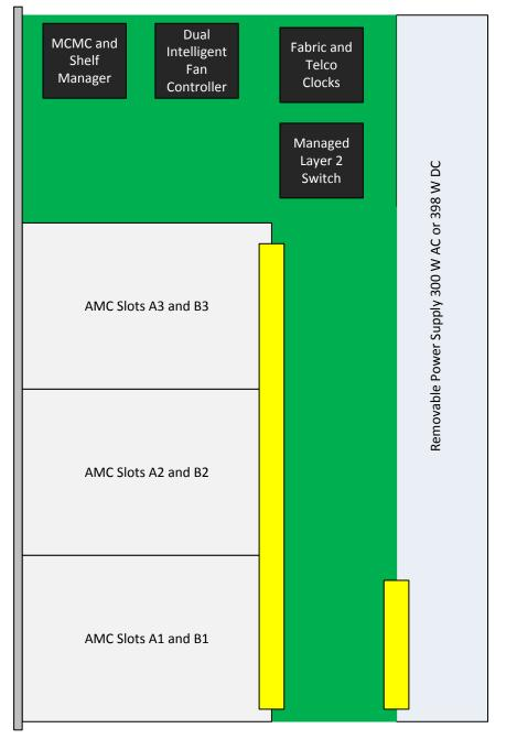
Figure 3: Top Level Block Diagram
