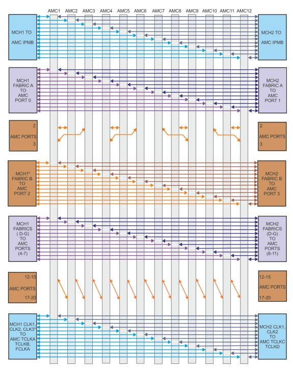
Figure 5: VT867 Backplane Connections
