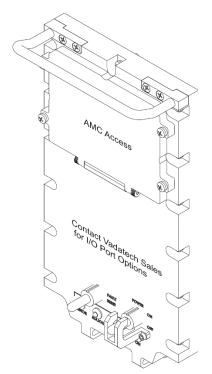
Figure 2: Front Panel Example with Access to I/O Ports Only
