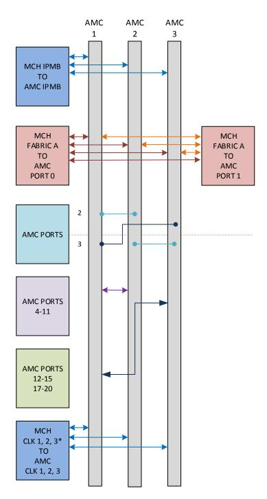
\* MTCA specifies three clocks CLK1, CLK2 and CLK3. The CLK3 can be routed to each AMC slots as Fabric clock (PCle clock or HCSL) or as Telco clock.
