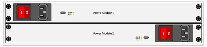
Figure 4: VT880 Chassis Layout
