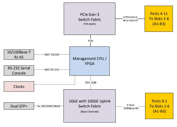
Figure 5: VT950 Block Diagram
