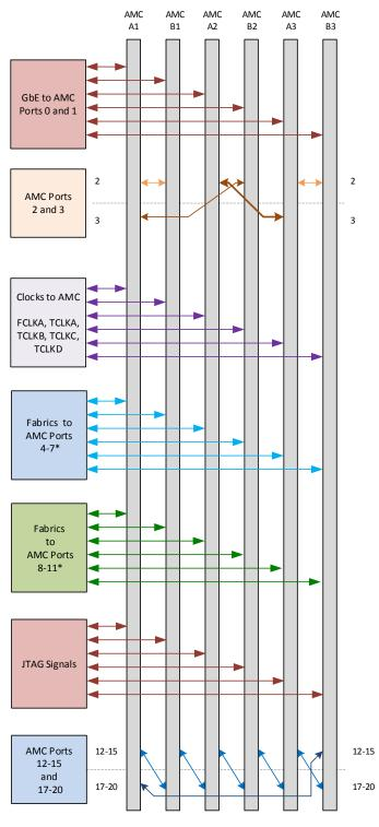
\*PCle Fabric can be configured to run as x8 bus (Ports 4-11)
