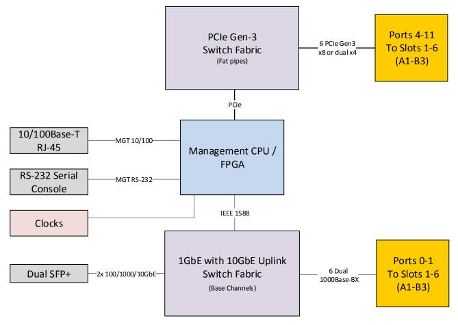
Figure 6: VT955 Block Diagram
