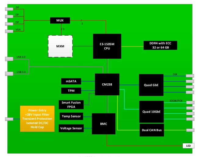
Figure 4: VT986 Functional Block Diagram
