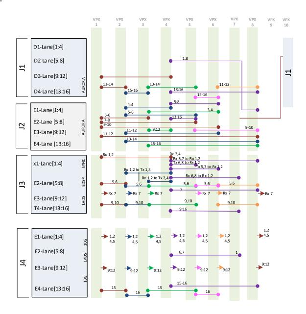
Figure 4: VTX351 Backplane Connections J1-J4
