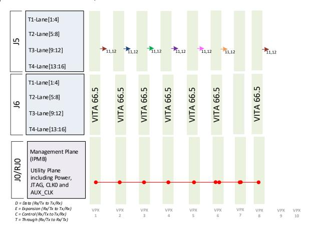
Figure 5: VTX351 Backplane Connections J5-J6 and J0
