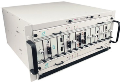
Figure 1: The VT866 was the first 40G MicroTCA chassis available in 2014.
