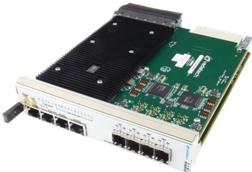
Figure 3: The UTC006 is a double module MCH with fabric options.
