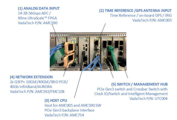
VadaTech provides support for the assembly of the module into a CuSTom (CST) integrated system with advanced functions. This system includes:
