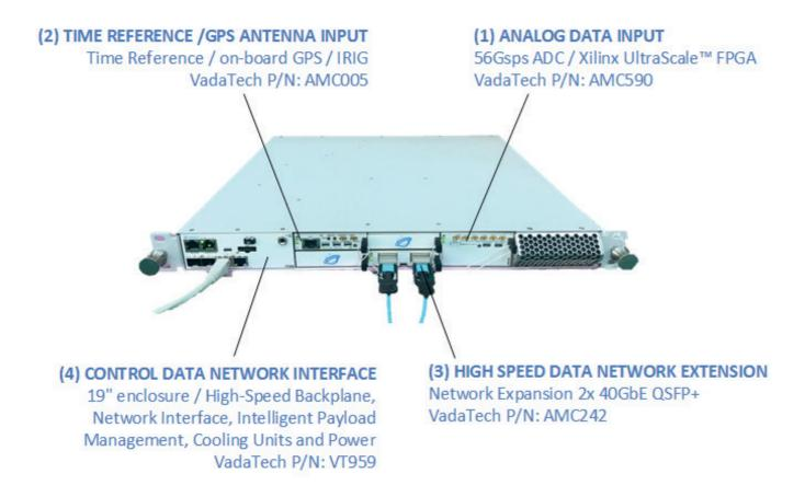
VadaTech solutions are based on a standard and modular architecture which allows to scale the solution and comply with the performances, size and budget available. Our customer needed a smaller footprint and tighter budget but required a higher network extension bandwidth for data processing in an external server. This deliverable allowed the customer to:
