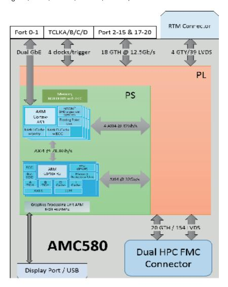
The Zynq Ultrascale+ MPSoC links the FPGA section to a complete compute unit, with a Quad-core ARM Cortex-A53, a Dual-core ARM Cortex-R5 and an ARM Mali-400MP2 Graphic Processing Unit.
