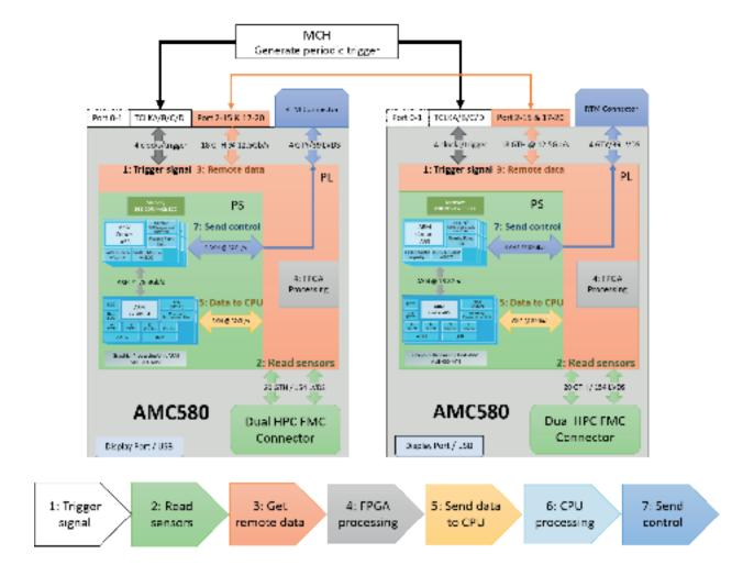
The AMC580 based system can have a total communication latency below 500ns. Which in this application case give a budget of 999.5us for the CPU and FPGA processing.
