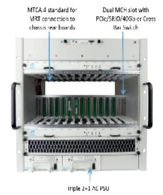
A Management Carrier Hub (MCH) includes the switches connecting up to twelve (12) boards together within one crate via the backplane. It also provides I/O and networking interfaces on its front panel. The MCH can be ordered with different switch options to match the protocol used to communicate between the boards in thte crate.
