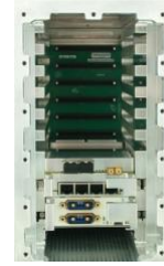
VT872 1/2 ATR Short, 6 AMC Conduction Cooled Chassis
