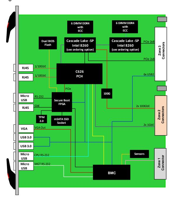
Figure 4: ATC129 Functional Block Diagram
