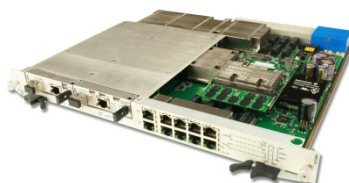
ATC806 40G/10G Switch w/Dual AMCs
