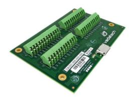
DA331 is a breakout module for the Oculink x4 cable style.
