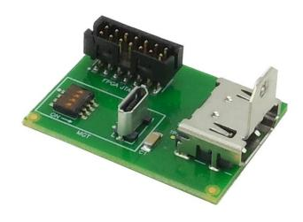
DA721 is a JTAG extender cable that enables standard JTAG pods to be used with VadaTech products fitted with a micro HDMI connector.
