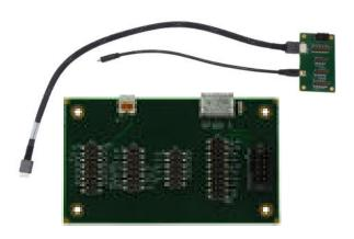
DA800 is a JTAG extender that enables standard JTAG pods to be used with VadaTech products fitted with custom pinout connectors. The adaptor board is supplied complete with Oculink and MicroHDMI cables.
