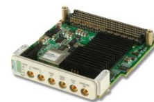
FMC210 ADC 10-bit 2.6 GSPS
